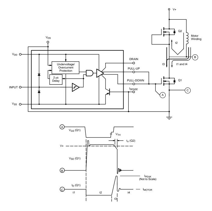
Figure 2. Clamping Inductive Flyback Energy
