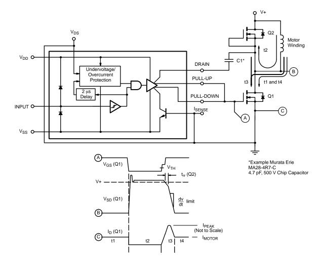
Figure 8. Direct dv/dt Limiting
