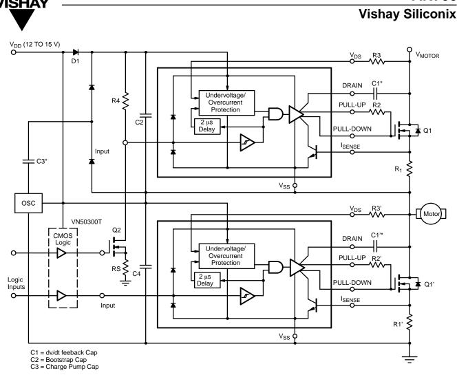
\*C1 - C3 0.3 to 1000 pF, 500 V, surface mount capacitors are available in a line of high Q porcelain ceramic capacitors from Murata.
