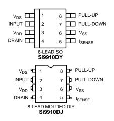
Figure 11. Si9910DY and Si9910DJ Package Pin-Outs
