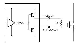
Figure 3. Simplified "Split" Emitter-Follower Output Circuit
