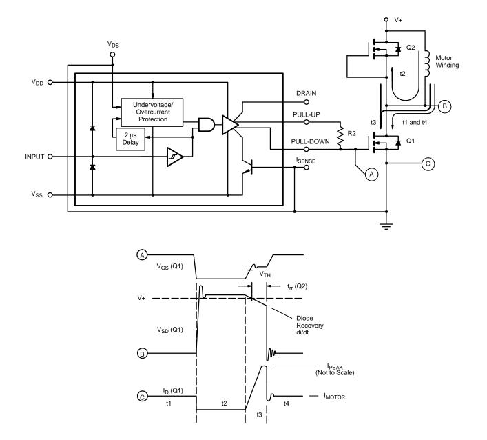
Figure 4. Controlling di/dt via MOSFET Gate Drive Impedance
