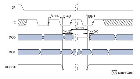
Figure 48: Output Timing
