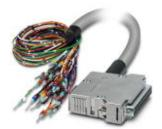
Assembled shielded round cable; connection 1: Single wires (37-position) (The wires are marked and fitted with ferrules. The braided shield is routed to a separate cable end.); connection 2: D-SUB socket strip (1x 37-position); cable length: 1 m
