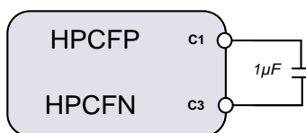
Figure 41: Charge Pump Flying Capacitor
