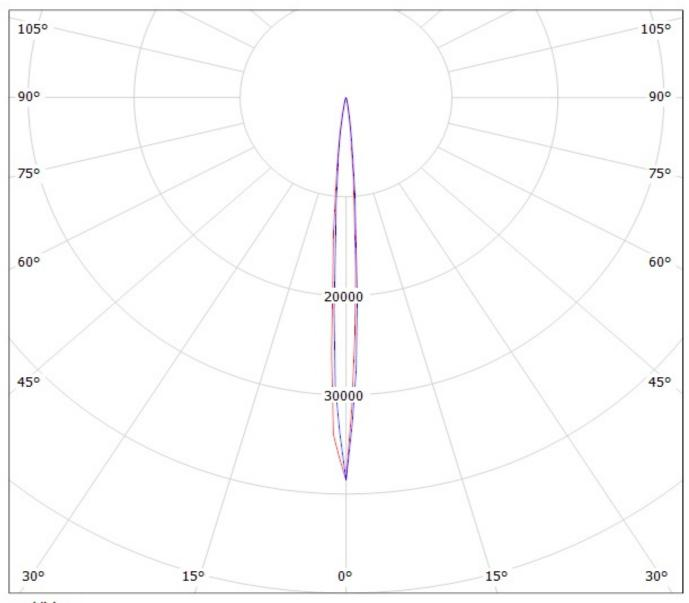
cd/klm \_\_\_\_\_\_ C0 - C180 \_\_\_\_\_ C90 - C270 Luminaire: Ledil Oy CP13059\_LOS-RS2 (Osram Square EC 69Im @ 250mA) Efficiency=92% Lamps: 1 x Osram Square EC 69Im @ 250mA
