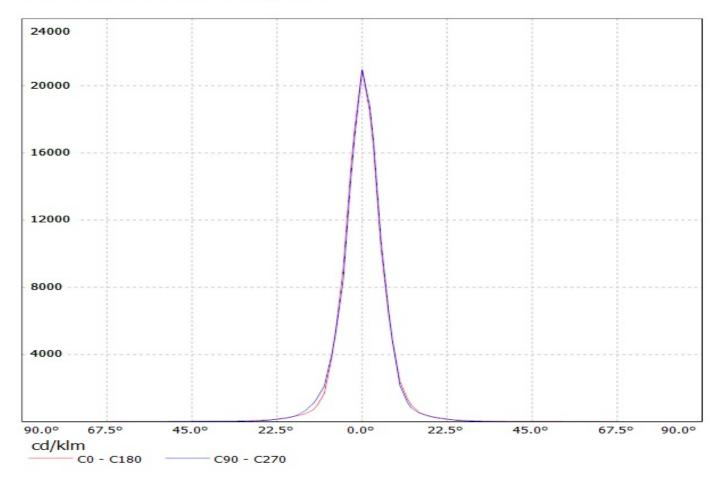
Luminaire: Ledil Oy CP13059\_LOS-RS2 (Osram Oslon 150dg 72Im @ 250mA) Efficiency=93% Lamps: 1 x Osram Oslon 150dg 72Im @ 250mA
