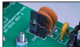
Figure 3. 110V jumper setting
