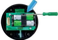
Replace the cover and tighten the (4) screws. Screws must be tightened to 5 in-lb torque in order to maintain IP66 rating. (This can be accomplished via hand tightening.)
