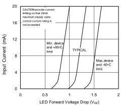
Figure 6. Input Characteristics (Current Controlled)
