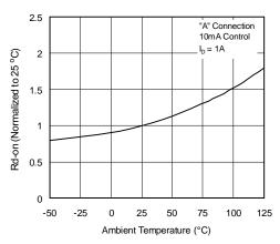
Figure 4. Typical Normalized On-Resistance
