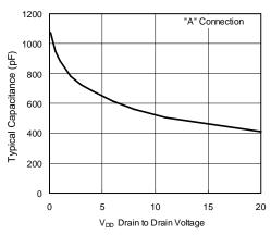
Figure 2. Typical Output Capacitance
