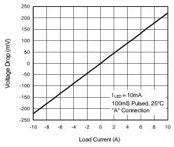
Figure 3. Linearity Characteristics
