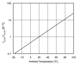
Figure 5. Typical Normalized Off-State Leakage
